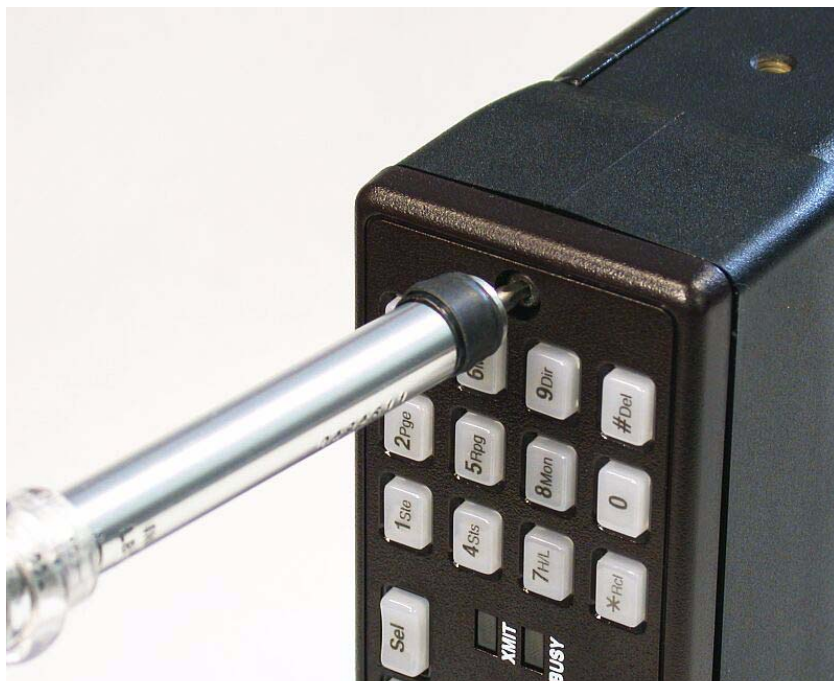
Figure 8-37. Installing the Control-Head Screws
