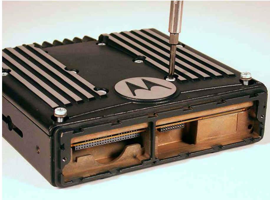
Figure 8-11. Removing the Top Cover Screws
