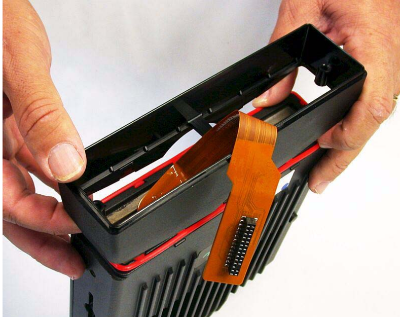
Figure 8-6. Removing the Headbridge
