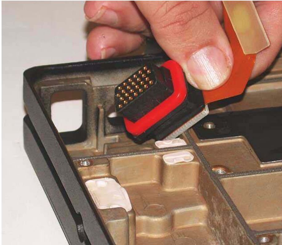
Figure 8-20. Removing the J2 Rear Accessory Connector
