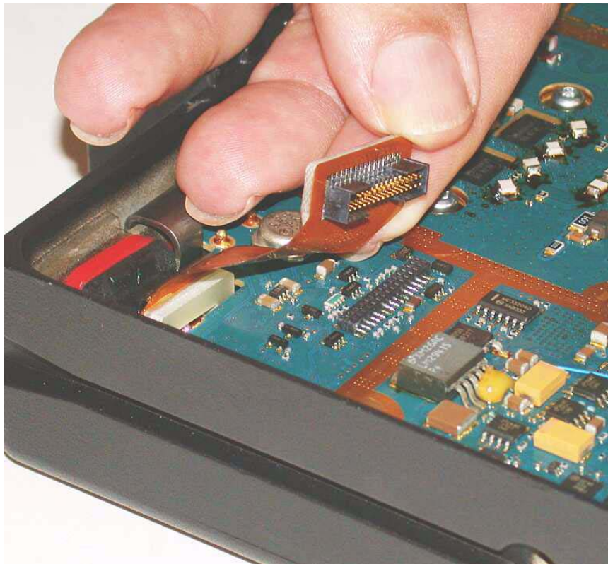
Figure 8-14. Removing the J2 Rear Accessory Flex from the Main Board
