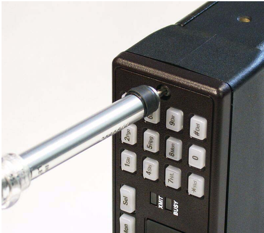
Figure 8-3. Removing the Front Panel Screws
